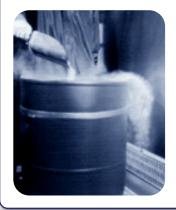
Sampling procedures can create clouds of powder, above the containment drum. A Containment Control System reduces the clouds and keeps the particulate free of contamination, and provides a safe environment for workers and other materials or products in the near-by vicinity.
